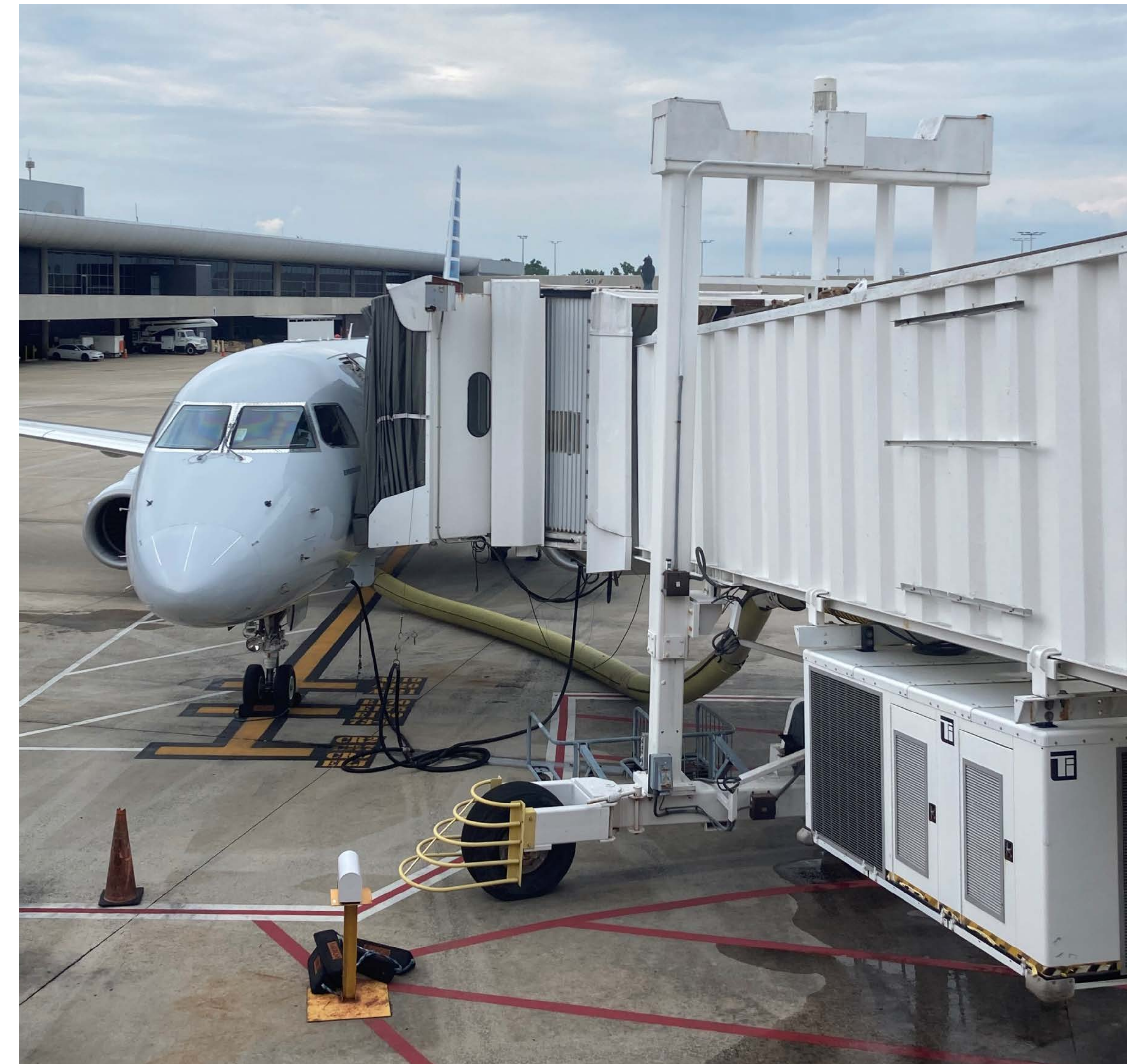
Ground Power Unit (GPU) at Gate 43
